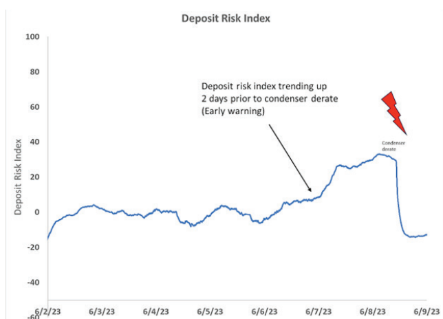
Figure 1. Plot showing deposit risk index at the power plant from the deposit sensor (higher the deposit risk index, higher the deposition stress). Deposit risk index trends up on 06/02/23 and 06/07/23 indicating increase in deposition stress during this period.
