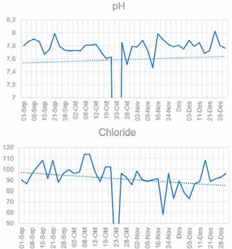
Figure 2. pH and chloride profile of cooling water during non-phosphate trial.
