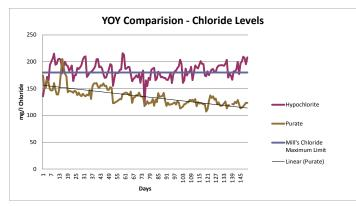
Figure 6 - YOY Chloride levels in the mill water - Before & after PURATE
